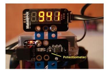
If you would like to check the angle of detection too, please move the candle and draw a line where the sensor loses the fire: in our case the angle resulted 40°.
