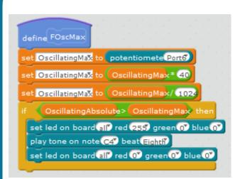
Here, we can see how the "OscillatingMax" variable collects the value of the potentiometer and sets the maximum value at which the mBot Ranger can incline.
