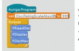
When we start the program, a default value will be set to the variable "OscillatingScaleAbsolute", which is the value of the Ranger angle indicator.
