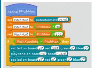
Here, we can see how the "PitchMax" variable collects the value of the potentiometer and sets the maximum value at which the mBot Ranger can incline.
