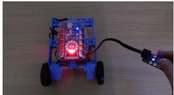
Proposition 2: All leds light in the same color, but the color is changing when the user spins the potentiometer
